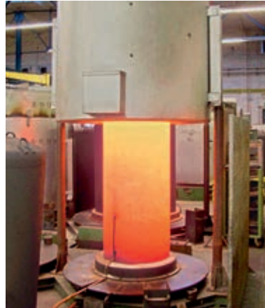
Bell furnace after removal of the heating mantle to start the cooling phase
