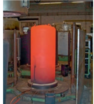
Bell furnace after removal of the heating mantle during the cooling phase
