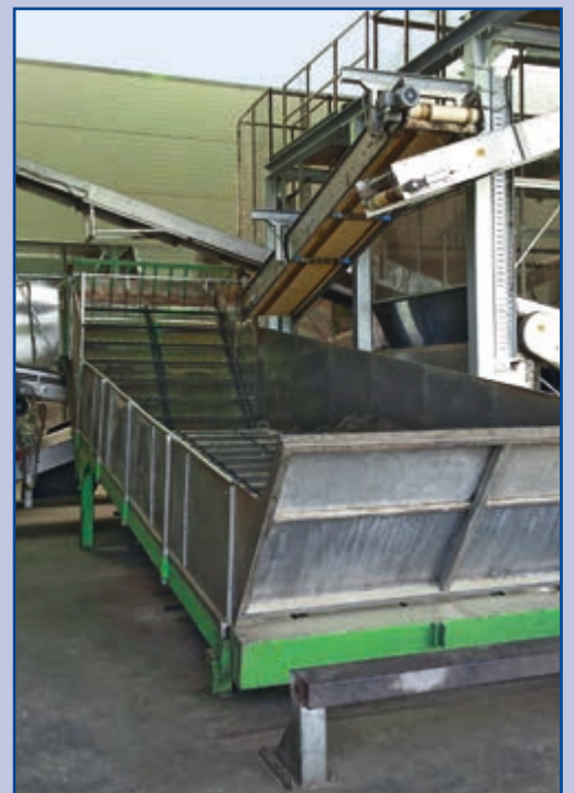
Inside view of the belt dryer
