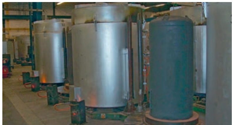
Bell furnace - without a heating mantle in the foreground, with a heating mantle installed in the background
